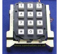
Most telephones use a standard keypad with 12 buttons or switches for the numbers 0 through 9 and the special symbols \* and #.
